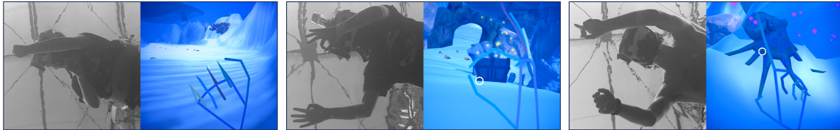
Figure 1: Participants used gestures with a waterproof head-mounted display to interact with a virtual underwater environment while submerged: grab for navigation (left), pinch for single actions (center), and point for continuous actions (right).
