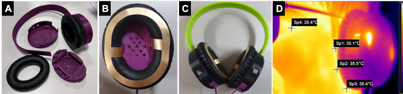
Figure 1: Thermoactive headphones for thermal comfort developed with low-cost materials (A), using Peltier elements and flex-printed metal plating for heat transfer (B&C), efficiently warming the user (D).
